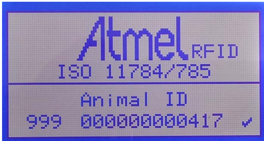
Figure 1-6. LCD Display with Animal ID Read Selection in Stand-alone Mode
