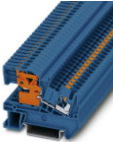
N disconnect terminal block, Push-in connection, Cross section: 0.14 mm 2 - 4 mm 2 , AWG: 26 - 12, Width: 5.2 mm, Color: blue, Mounting type: NS 35/7,5, NS 35/15
