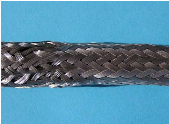
NOT ACCEPTABLE Uneven Coverage
