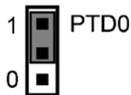
Figure 7-11: Accelerometer g-Select1 Jumper settings (J13)
