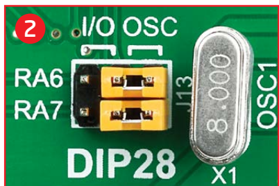
Figure 4-7: RA6 and RA7 connected to X1 quartz-crystal
