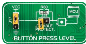
Figure 10-5: Button press level jumper (J17)
