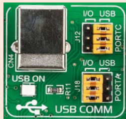
Figure 8-2: USB enabled on PORTC
