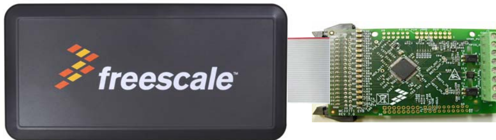
Figure 6. BATT-14AAAPACK Connection to KIT33771TPLEVB
